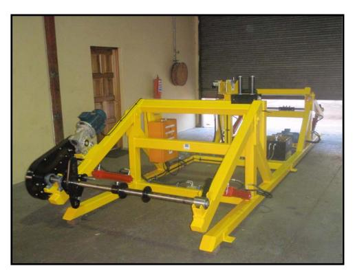
The 5 ton coiling and winding machine is the mid range level for automated cable winding and coiling operations. This machine is perfect for operations requiring speed, minimum labour and handling of volume based operations.
